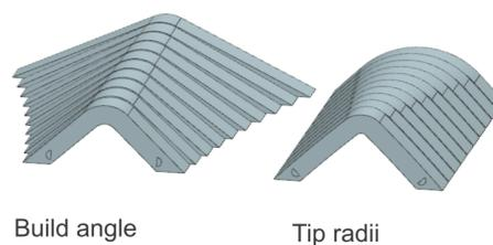
**Figure 4. Model of design artefacts developed by one company to evaluate the need for support structure.**
