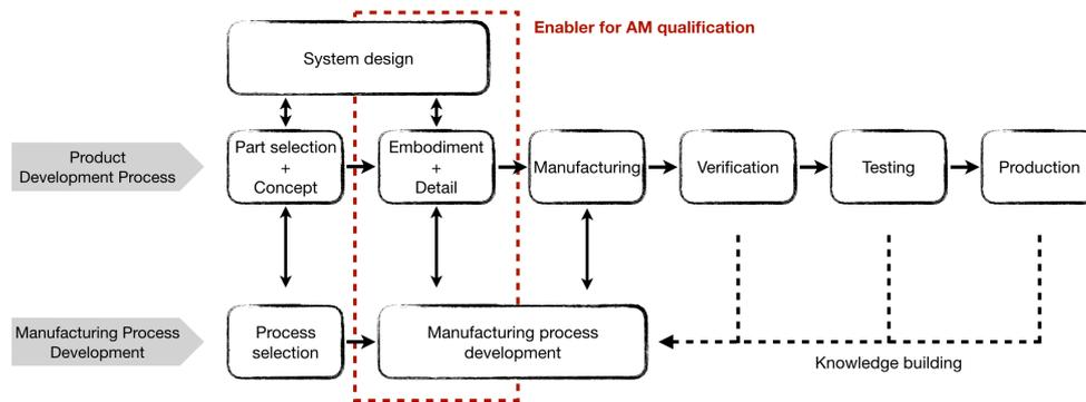
**Figure 1. Refined model of the product development process for AM in space applications, utilising concurrent product and manufacturing process development and systems design (Dordlofva, 2018).**
