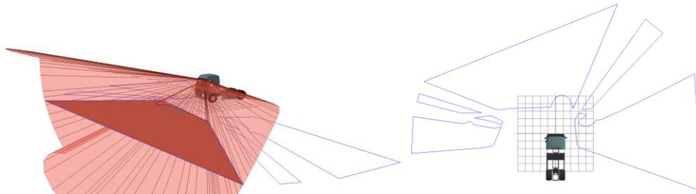
Figure 5. 3D Field of View Projection clipped to the ground plane to form 2D ground plane projections for direct vision
