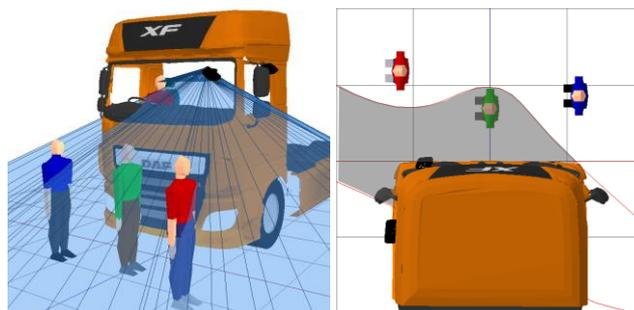
*Figure 11. The configuration of the pedestrian models positioned in front of the vehicle for indirect vision analysis. The image to the left shows a 3D view to Class VI mirror projection. The image to the right shows a plan (top-down) view.*
