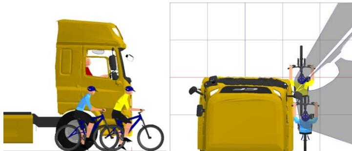
Figure 9. Cyclist models positioned to the driver side of the vehicle.
