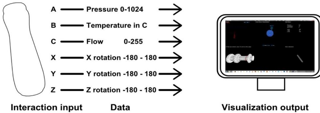
Figure 5. Diagram shows the connections between the TUI and GUI that consist of six different values and their individual ranges. An Arduino captures the data from the various sensors.
