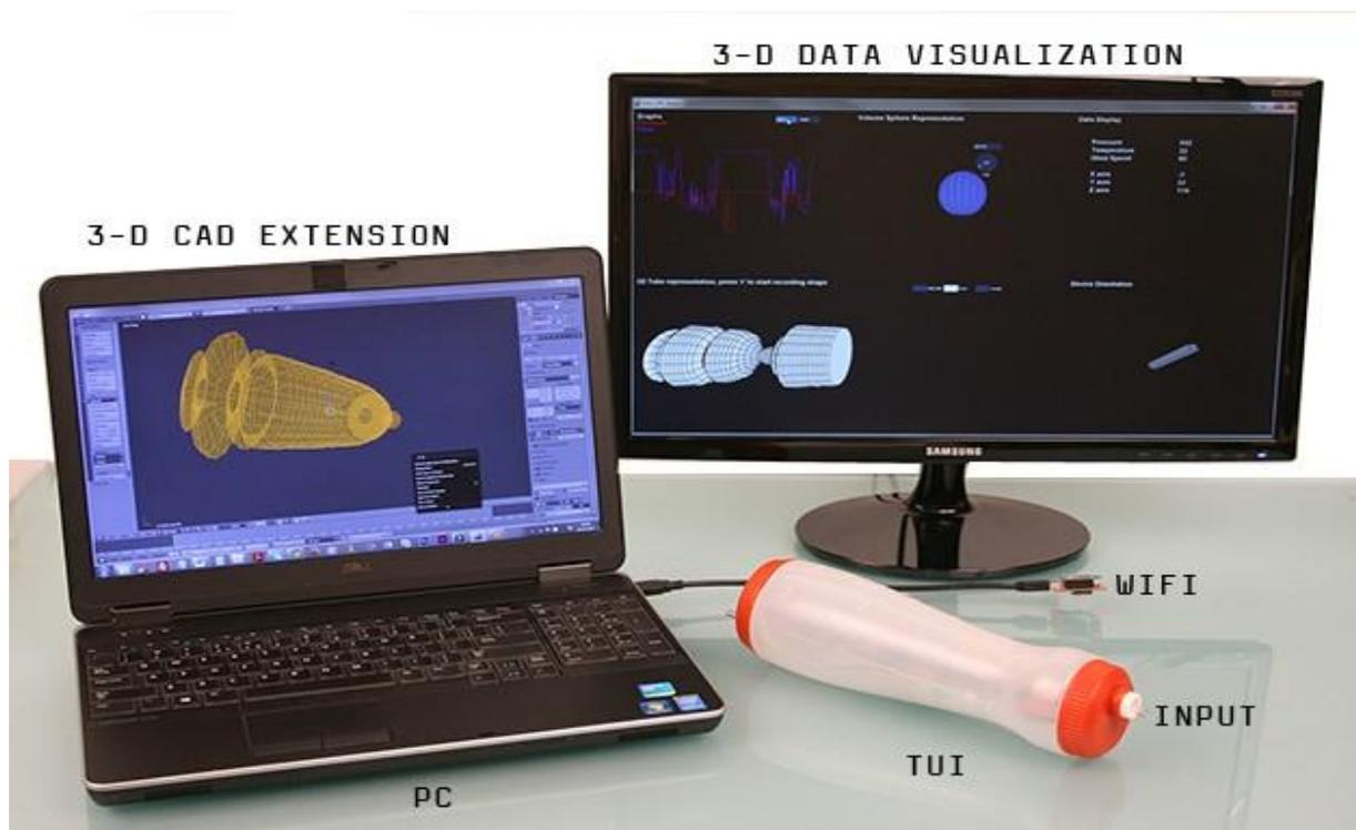
Figure 4. AFIF complete setup; shows pc with Blender visualization of generated content (3-D CAD), 3-D data visualizer of blow IA and tangible user interface (TUI) in foreground right.
