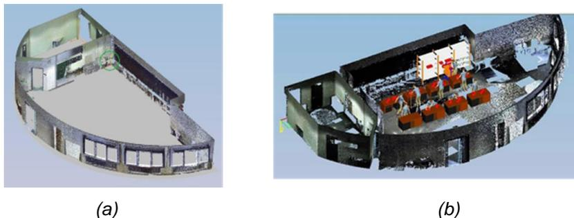
Figure 8. (a): integrated ground plane; (b): CAD generated assembly stations in the point cloud environment
