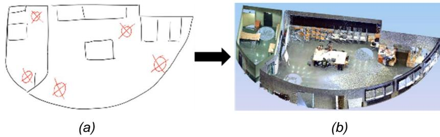
Figure 7. (a): two-dimensional layout draft of scan positions, (b): related point cloud data
