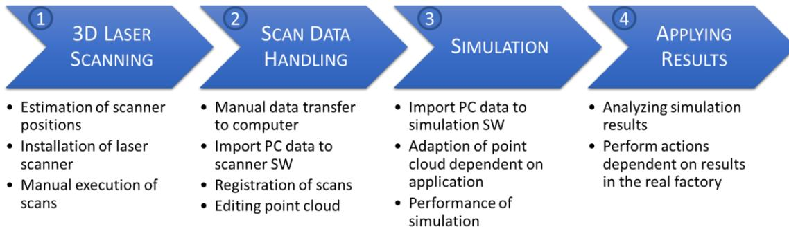
Figure 2. State of the art process of performing a simulation based on point clouds
