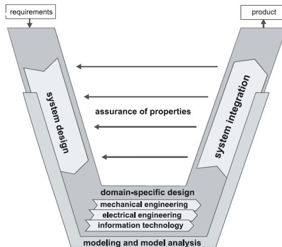
Figure 5. The V-Model according to guideline VDI 2206 (VDI, 2004; Gausemeier and Moehring, 2003)
