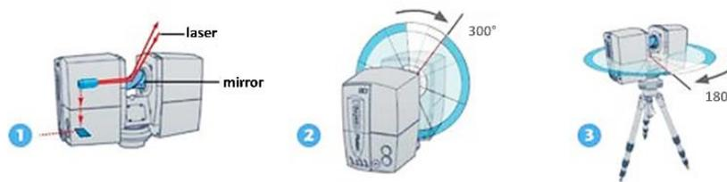
Figure 1. The functionality of terrestrial laser scanners (Function Laser Scanner n.d.)
