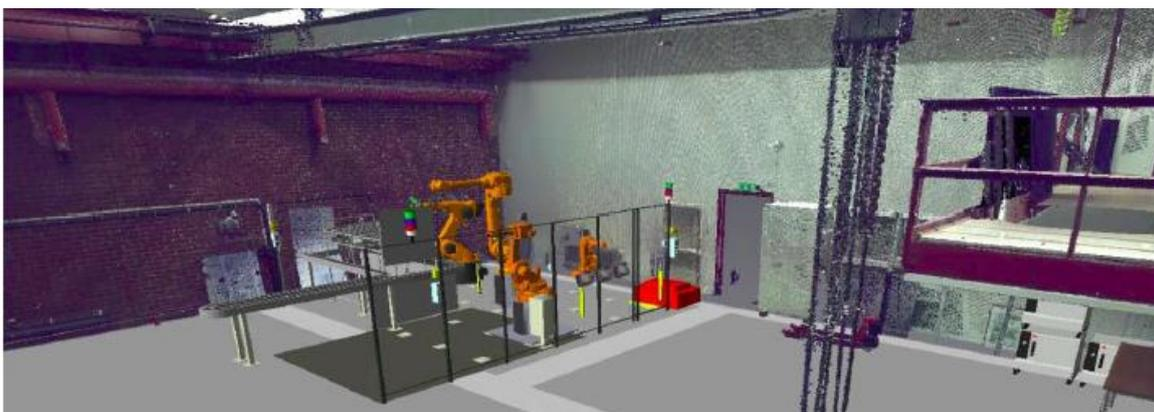
Figure 3. An example of 3D-models in a point cloud environment within a digital factory
