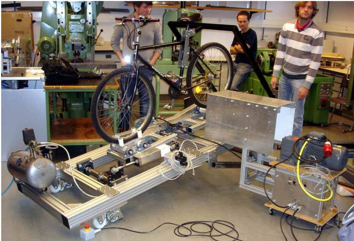
**Figure 2: Test device for bikes**
