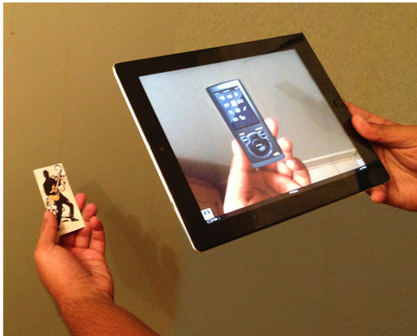
Figure 5. The Layar Application detecting the marker graphic and placing the 3D model and HTML/Java Script interaction on top of 3D model.
