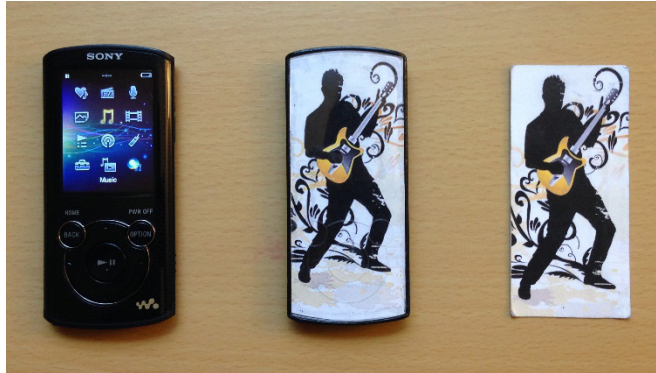
Figure 6. Usability testing using actual product (Non-AR, Left), 3D printed model with a marker card pasted on it (AR1, Center) and marker card (AR2, Right).
