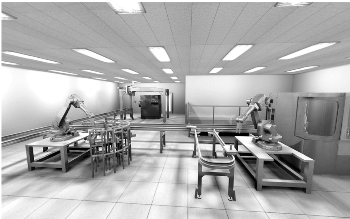
Figure 3. Overview of the monorail conveying system with proper processing stations and robots
