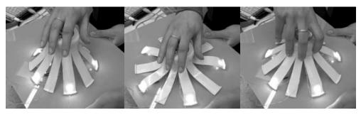
Figure 3. This successful hack exploits a cut-up plastic cup both as a spring and as a light diffuser
