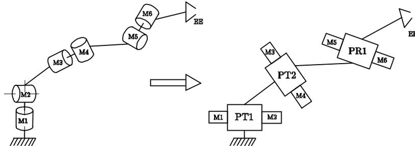
Figure 2. Proposed 6-dof hybrid manipulator
