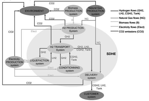
Figure 5. Presentation of the system of distribution of hydrogen energy (extracted from [10])
